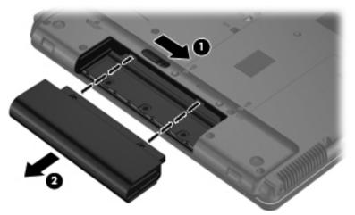
Install the battery by inserting it into the battery bay until you hear a click.
